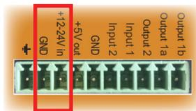
It is recommended to connect the earth ground in order to reduce interference of noise.
