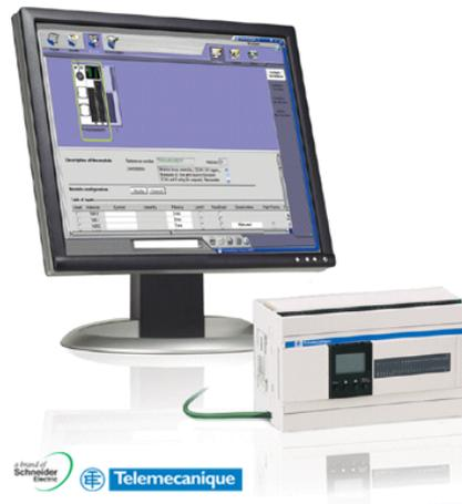
5. the Twido Suite will now search the installed COM ports on the computer for the PLC (A COM port in this case is mapped to a USB driver)
