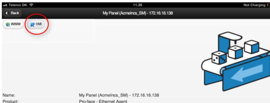
**NOTE:** If the HMI button does not appear, it means the remote HMI application has not been installed or activated on the panel, or the SiteManager has a firmware version older than 5.6 build 14265.
