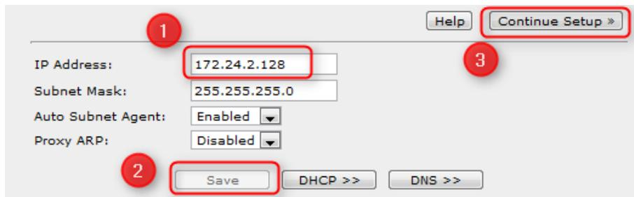
**Hint:** If your device is configured to receive an IP address from a DHCP server, you could have enabled DHCP in this menu, which would make the SiteManager act as a DHCP server that assigns IP addresses to devices on the DEV network.
