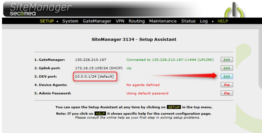
31. The PLC in our example has IP address 172.24.2.129/24 (/24 means it has subnet mask 255.255.255.0). So the address for the DEV port must be a free address in this subnet (172.24.2.x) , for instance 172.24.2.128.
