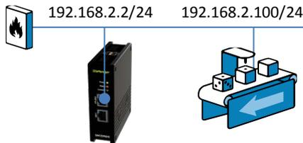
**NOTE:** The machine depicted represents the network device you want to use as "remote monitored device" for this exercise. You can, however, use any IP enabled device, such as a PLC, HMI or even a PC or a printer. In the following we are using a PLC attached on the DEV side of the SiteManager.
