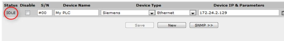
**Hint:** If it does not go idle, it means the SiteManager does not get a response from the device, and you should check the configured IP addresses and Ethernet wiring again.
