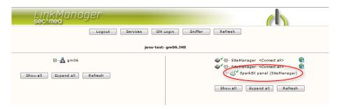
2. When connecting the agent, you should see some activity in the tray icon area, which is the auto configuring of a virtual serial port. If your SiteManager, and the UniOP eTOP HMI is correctly attached, you should also see the status of the agent become OK, and a few bytes of traffic:
