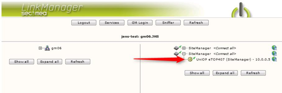
2. You will not see any activity on it yet. This only starts when you connect to the PLC via your project (Make a note of the IP address of the HMI):
