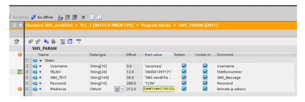
Make sure that the telephone number to receive the SMS is correct and the Remote IP address is set to the SiteManagers DEV IP address.
