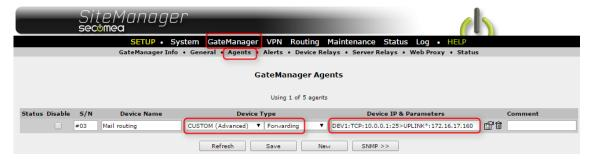
Note that the SMTP server may limit access to specified devices or IP addresses. So you may have to apply the Uplink Source Translation parameter (+TUP) to the forwarding rule, which will source NAT the connection and let the SMTP server allow access for the SiteManager's Uplink address as source for the mail connection.
