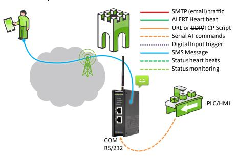
With a serial connection (RS232) between the PLC and the SiteManager you can use the SiteManager as serial modem on which you can read incoming SMS messages using the standard AT-command set.
