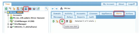
Select a meaningful name for the Alert, as this will become the Alert message text. You can now specify for instance to trigger the alert when Input2 is ON.
