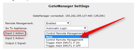
**Note:** You can also change it to Trigger Input1 if ON/OFF, which will make the trigger also appear on the GateManager, where it can be controlled by the "GateManager controlled Alerts" ref. section 8. This will not affect the functionality for the local Alert you have configured for Input1.
