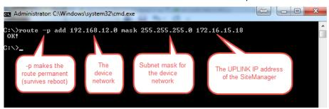
Then configure your software to access the IP address of the devices directly. le. 192.168.12.4 and 192.168.12.5.
