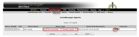
In this example Routing is allowed for the addresses 172.16.16.223 and 172.16.16.225. You can define a maximum of three devices.
