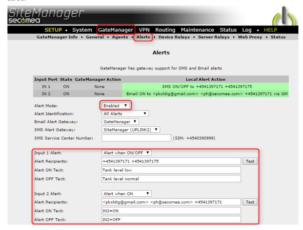
**Input Alert state** – Enable and set the state of the input alert to be triggered. State can be ON, OFF or both.
