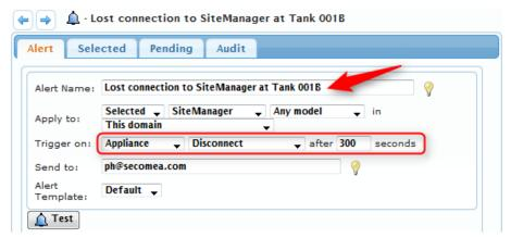
Note in this example that the Alert is not triggered until after 300 seconds. This will ensure that e.g. a brief repower of the SiteManager at the location will not activate the Alert.
