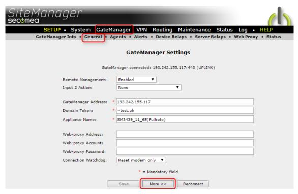
Now you can control for both Input1 and 2 when a signal should be sent to the GateManager based on triggering of Input 1 or 2.
