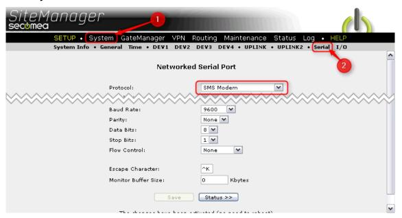
**NOTE:** When enabling SMS Modem, the Serial port <u>cannot</u> be allocated a Serial agent
