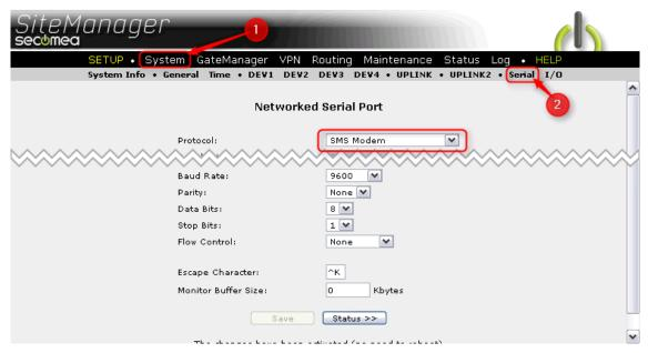
NOTE: When enabling SMS Modem, the Serial port  $\underline{\text{cannot}}$  be allocated a Serial agent
