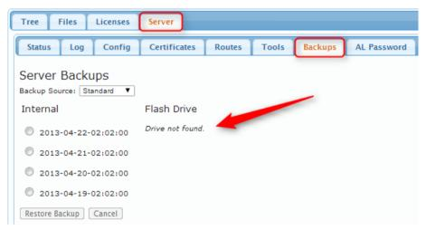
When inserting a properly formatted USB drive, this page will display the default backup intervals:
