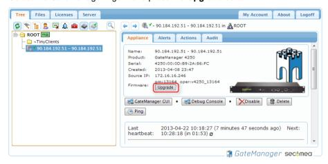
5. Press the Upgrade button for the newly uploaded firmware.
