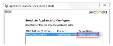
As a security precaution the GateManager will prevent access by the Appliance Launcher after 10 minutes, so that it will not be interrupted during normal operation.
