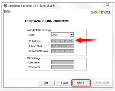
**NOTE:** If you intend to relocate the GateManager to a network without a DHCP server (such as a firewall DMZ), you should define a static IP address and the Default Gateway through which the GateManager can access the Internet.
