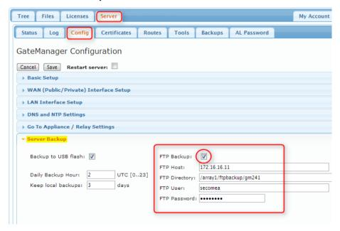
**Note:** If no USB drive is attached to the server you should uncheck the option "Backup to USB flash:" Leaving it checked will result in the logon splash screen saying "Last Server Backup failed".
