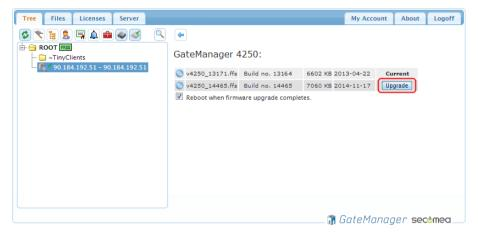
6. While upgrading *Upgrade in progress* is shown on the screen. The upgrade will usually take less than 60 seconds.
