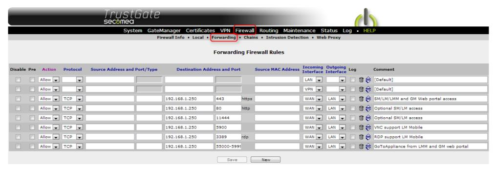
• You could decide to replace the first rule that allow full access from the LAN to the Internet, with specific ports required by the GateManager according to the list of outgoing port in section **3.1 Configuring your corporate firewall**.
